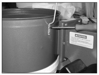
Figure 10. Installing upper bag support.
